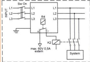
In case of phase loss relay 4 opens after a delay time of 30ms. Synchronic the relay of the appropriate phase opens, too and its green LED extinguishes. When the phase sequence is incorrect, relay 4 opens after a delay time of 30ms. The Phase Error LED lights red. When the phase sequence is correct the LED is off and the relay 4 is closed.
