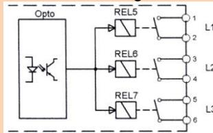
Relay 5 to 7 are galvanic insulated via opto-couplers. If L1 to L3 are operating the relays are closed. If one phase drops its relay opens and the message can be used with an active signal (60V/500mA maximum load each relay).
